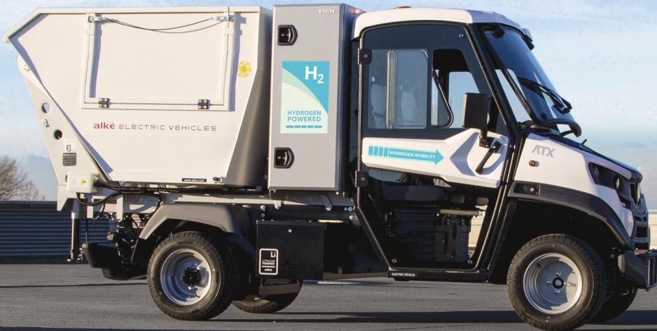
The Alkè ATX electric vehicle with hydrogen range extender is 100% eco-friendly, high-performing and extremely robust. FCH technology, combined with the lithium battery, guarantees a range increase of 160 km. This vehicle represents an innovation
